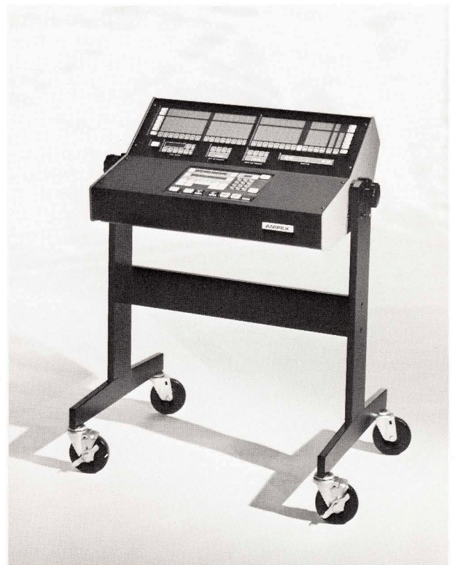
Figure 2. A roll-around pedestal containing the channel function and multi-point search-to-cue modules.
